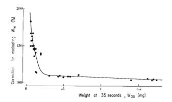
Fig. 4. Correction applied to fibers weighed 35 seconds after their removal from the solution
