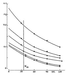
Fig. 2. Weight change in 6 small fibers due to evaporation. The fibers were not blotted and the weights so obtained ranged between 0.1 and 0.3 mg. Curves are extrapolated back to zero time. The time axis is in seconds after removal of the fiber from the solution
