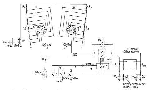
Fig. 1. Schematic diagram of the integrative flame photometer. Simultaneous with the insertion of the sample-bearing platinum loop into the flame, a synchronizing pulse initiates the relay closure for a predetermined interval. As the sample burns, the signal is recorded, and its integral (the condenser voltage) is measured by the Keithley electrometers. When the platinum is withdrawn, the condensers are discharged
